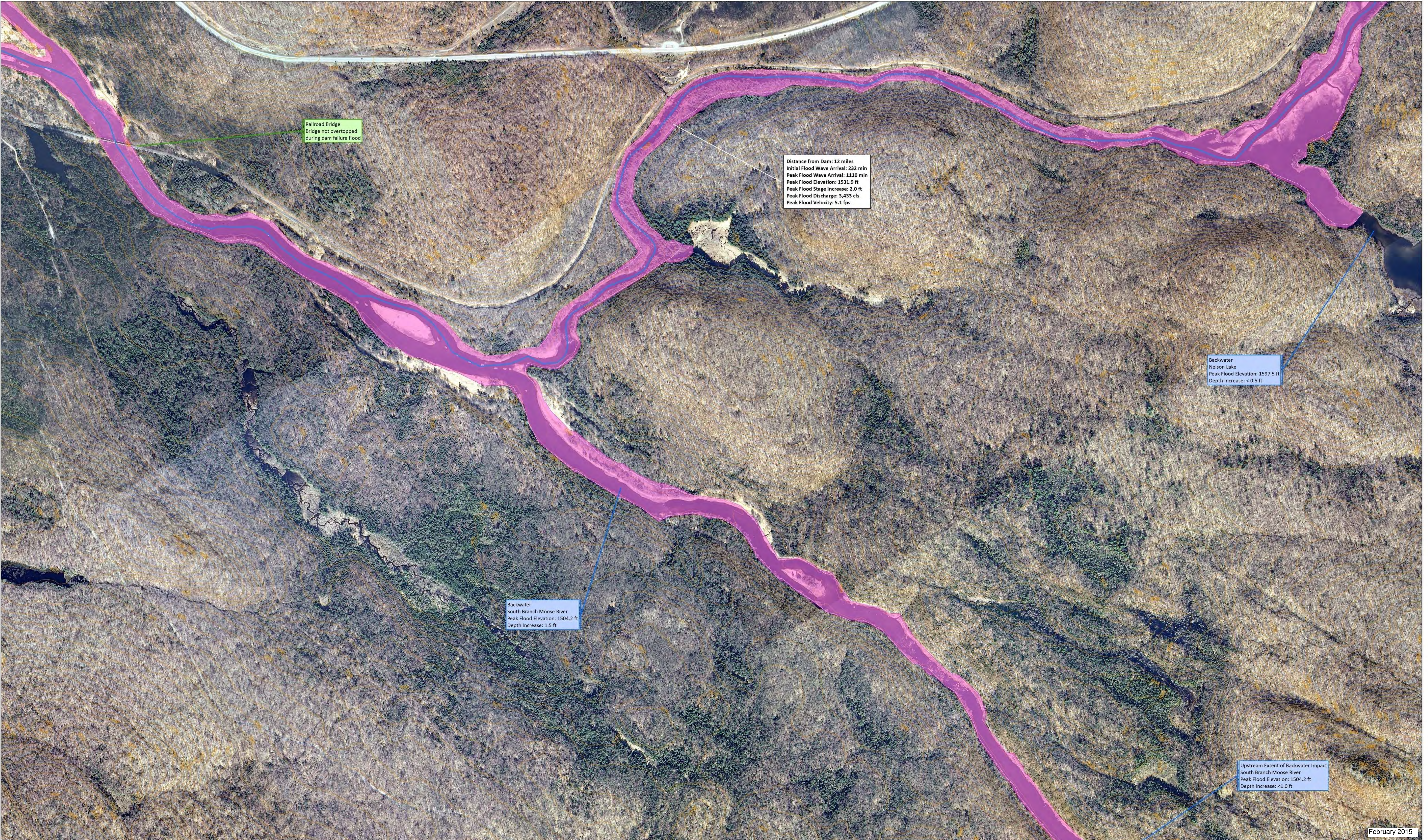
Figure 7-10 Old Forge Dam Emergency Action Plan Dam Failure Inundation Limits "Stormy Day" Scenario
